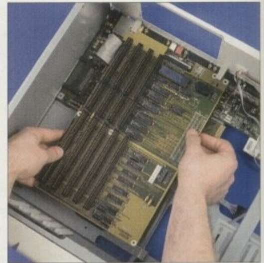
With the A1200 motherboard in position and securely screwed down, the Zorro slot busboard is plugged onto the motherboard via the adapter
